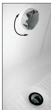
Rotate the handle counter-clockwise to open the dewater valve; otherwise, shut it. When the water is higher than maximum level, the surplus will split out through sewer pipe.
